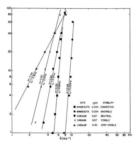
Figure 6.5 Comparison of observed wind speed profiles at different sites ( $z_{\theta}$  is a measure of the surface roughness) under different stability conditions with the power-law profile. [Data from Izumi and Caughey (1976).]
