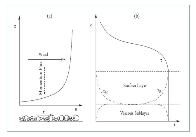
Fig. 5.4. (a) An illustration of mean wind profile in the surface layer. A downward momentum flux corresponds to shear stress in the direction of the wind. (b) Profiles of effective shear stress, , Reynolds shear stress,  $\tau_R$ , and viscous shear stress,  $\tau_m$ . In the surface layer,  $\tau = \tau_m + \tau_r$  is approximately constant.
