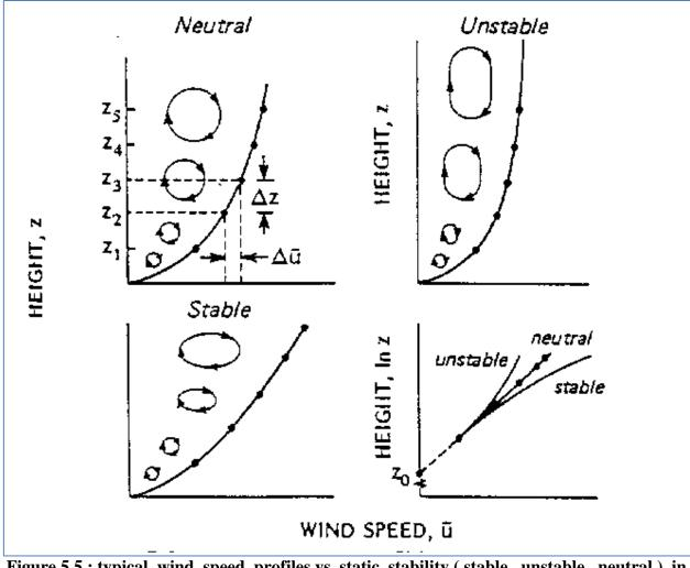
Figure 5.5 : typical wind speed profiles vs. static stability (stable, unstable, neutral) in the surface layer
