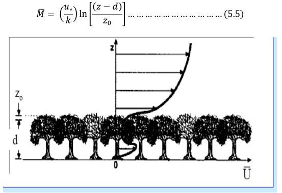
Fig(5.3) :flow over forest canopy showing wind speed, M, as a function of height z.
