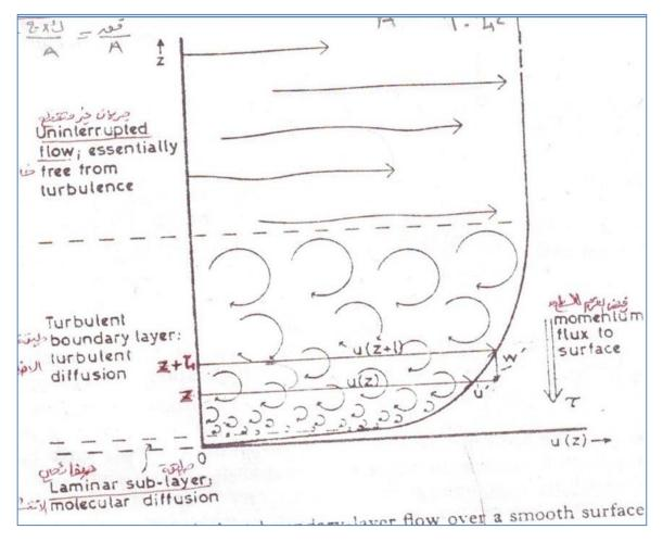
Figure (5.1): Turbulent -boundary -layer flow over a smooth surface.
