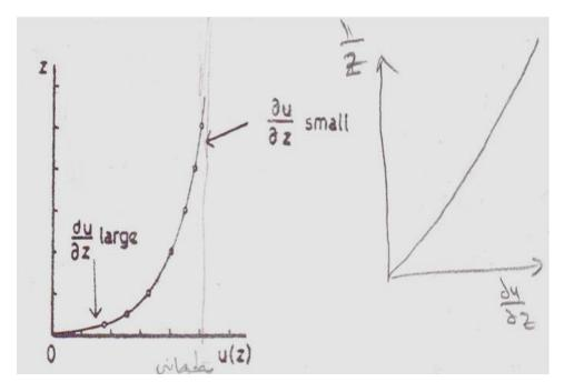
Figure (5.2) : typical wind profile over a uniform surface .
