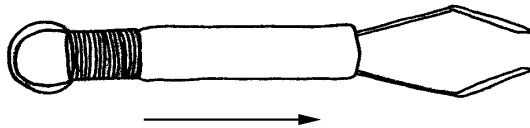
Figure 5: Small pair of curved forceps or tweezers made of metal. The middle section is movable and can be moved back and forth to open and close the tweezers.
