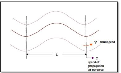
Since the last term in the equation  $(\frac{\beta L^2}{4\pi^2})$  is always positive, the wave speed C must be smaller than the wind speed. Thus, the air passes through the troughs and ridges at a speed greater than the pattern itself propagates.
