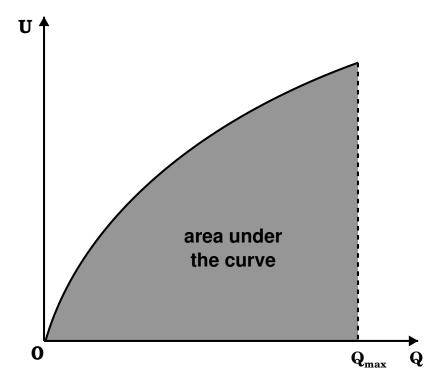
c) The integration starts when the capacitor is discharged: U = 0 and Q = 0 and continues until the maximum charge is reached  $Q \Longrightarrow Q_{\text{max}}$ :
