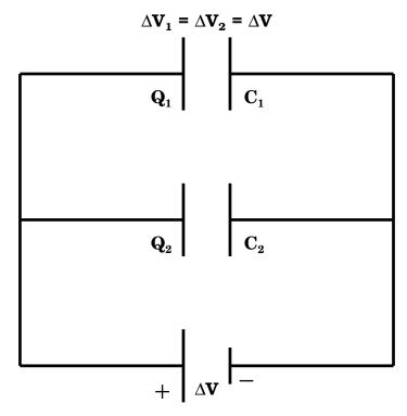
a) In parallel, we can reduce the diagram above to the following diagram:
