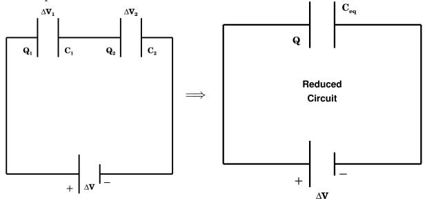
a) For a series combination of capacitors, the magnitude of the charge must be the same at all plates:
