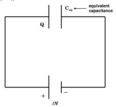
b) The potential difference across the capacitors  $\Delta V_i$  in a parallel circuit are the same  $\Longrightarrow$  each is equal to the battery's voltage  $\Delta V$ .
