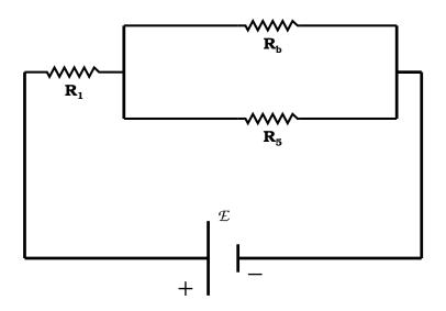
The diagram below show the next stages on route to the final equivalent resistor: Reduce the parallel  $R_b$  and  $R_5$  resistors followed the series  $R_c$  and  $R_1$  resistors as shown in the next diagram.
