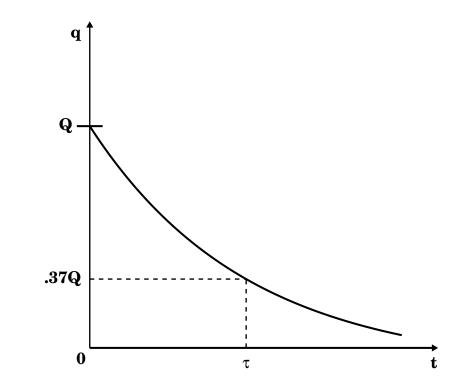
c) Note that the capacitor is now acting like a battery, however, a battery with a continually decreasing voltage:
