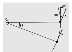
Fig. 6.1 Centripetal acceleration is given by the rate of change of
