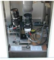
This disdrometer uses two, side video to record optical images of each raindrop.
