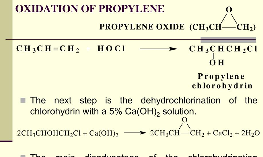
The main disadvantage of the chlorohydrination process is the waste disposal of CaCl<sub>2</sub>.
