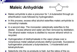
Selectivity into the co-products is high, but the ratios of the coproducts may be controlled with appropriate reactor operating conditions.
