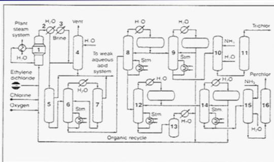
The PPG Industries Inc. Chloroethylene process for producing perchloro and trichloroethylene: (1) reactor, (2) graphite exchanger, (3) refrigerated condenser, (4) scrubber, (5) phase separation of perchloro from trichloro, (6,7) azeotropic distillation, (8) distillation train, (9-11) crude trichloro separation - purification, (10-16) crude perchloro separation - purification.
