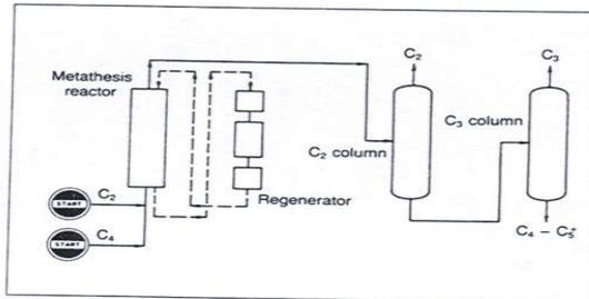
A flow diagram showing the metathesis process for producing polymer grade propylene from ethylene and 2-butene.
