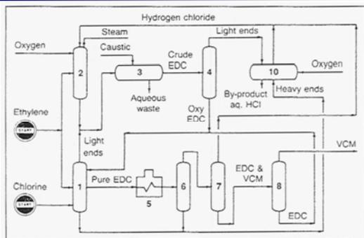
The European Vinyls Corporation process for producing vinyl chloride: (1) chlorination section, (2) oxychlorination reactor, (3) steam stripping and caustic treatment of water effluent, (4) EDC distillation, (5) pyrolysis furnace, (6,7,8) VCM and EDC separation, (10) By-product reactor.
