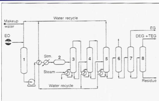
The Scientific Design Co. process for producing ethylene glycols from ethylene oxide: (1) feed tank, (2) reactor, (3, 4, 5) multiple stage evaporators, # 4 operates at lower pressure than # 3, while # 5 operates under vacuum, evaporated water is recycled to feed tank, (6) light ends stripper, (7, 8) vacuum distillation columns.
