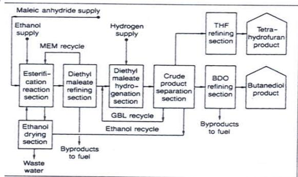
A block diagram for producing 1,4-butanediol from maleic anhydride
