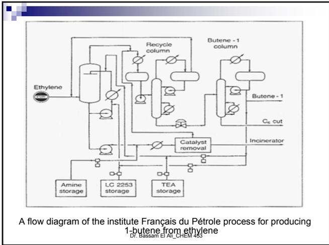
A flow diagram of the institute Français du Pétrole process for producing 1-butene from ethylene
