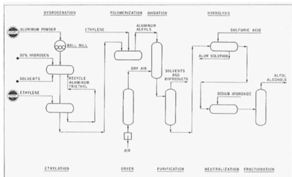
The alfol process for making even numbered straight chain alpha alcohols
