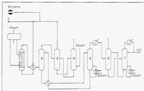
The Scientific Design Co. Ethylene Oxide process: (1) reactor, (2) scrubber, (3,4) CO<sub>2</sub> removal, (5) stripper, (6,7) fractionators.
