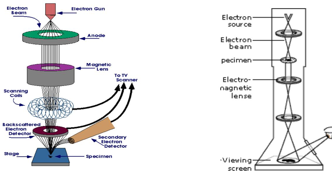
Figure (1) A. Scanning Electron microscope B. Transmission electron microscope
