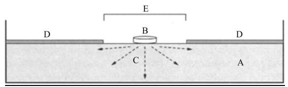
Disk sensitivity test. A – agar; B – antibiotic disc; C – antibiotic diffuses into agar along concentration gradient; D – bacterial growth on surface of agar after 18 hours of incubation; E – zone (diameter) of inhibition.
