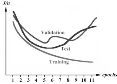
Fig. 6.19 A typical learning curve. The average error per pattern is plotted as a function of the number of epochs
