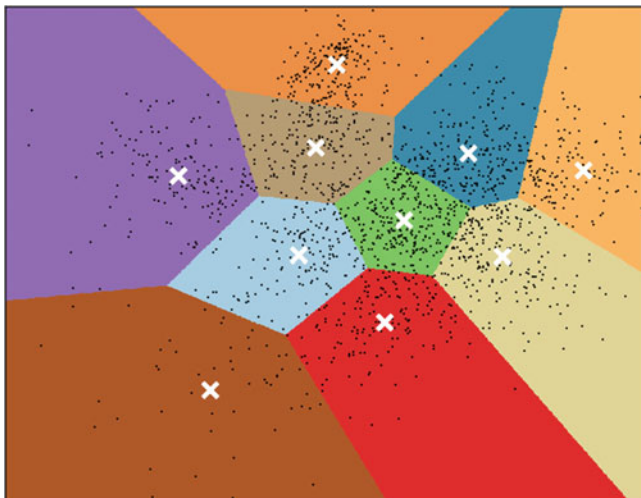
Fig. 8.5 The result of k -means clustering on handwritten digits data (The centroids of the clusters are marked with a white cross, and the Voronoi cells for each cluster are colored)
