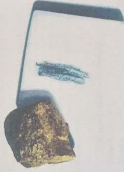
FIGURE 2.11 Although the color of a mineral is not always helpful in identification, the streak, which is the color of the powdered mineral, can be very useful (Photo by Dennis Tasa)
