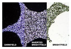
the objective and forms the image. This results in a specimen that is brilliantly illuminated on a dark field, The field surrounding the specimen appears black.
