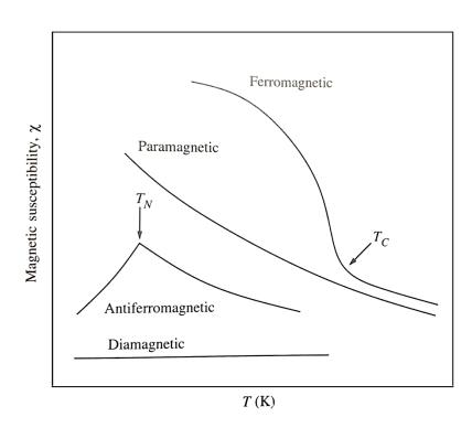
Variation of magnetic susceptibility with temperature for diamagnetic, paramagnetic, ferromagnetic, and antiferromagnetic substances. Transitions to paramagnetic behavior for ferromagnetic and antiferromagnetic and antiferromagnetic substances occur at the Curie  $(T_C)$  and Neel  $(T_N)$  temperatures, respectively.
