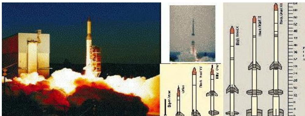
Rockets measure profiles of ozone levels from the ground to an altitude of 75 km by using photospectroscopy. Rockets provide all weather capability, but are limited by their short life and narrow geographic range. General info on [rocket probes](#).
