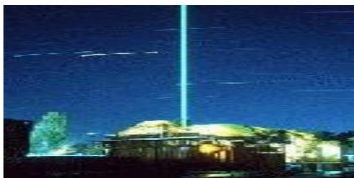
Light Detection and Ranging (LIDAR) is an ozone measurement technique that relies on absorption of laser light by ozone. A telescope is used to collect ultraviolet light that is scattered by two laser beams - one of which is absorbed by ozone (308 nm) and the other is not (351 nm). By comparing the intensity of light scattered from each laser, a profile of ozone concentration vs. altitude is measured from 10 km to 50 km.
