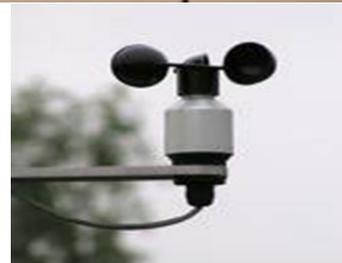
**Aerovane** – measures wind speed and direction
