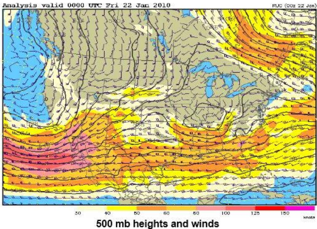
In curved flow, another force comes into play – centrifugal force (results in gradient wind balance)
