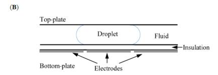
The figure above shows two droplet open microfluidic configurations (A) continuous flow emulsion-based droplet (from T-junction and flow focusing) (B) electrowetting-based droplet.
