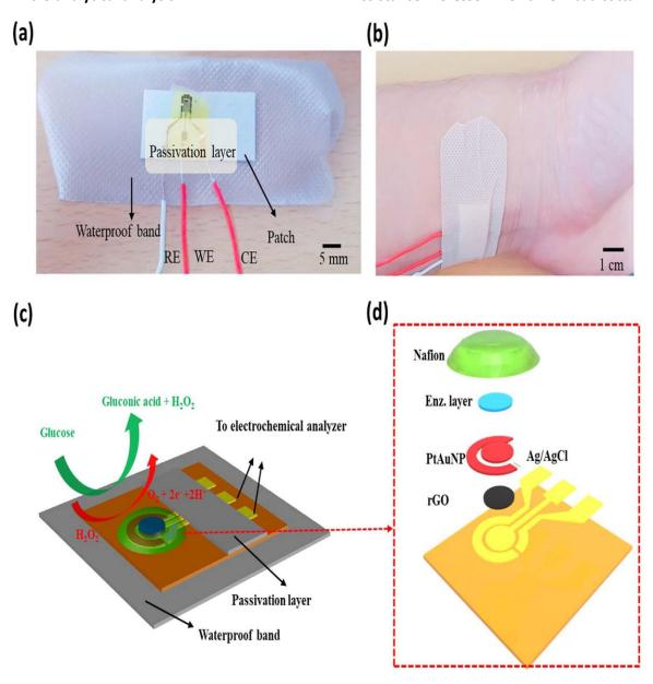
Photographs and schematics of the fabricated wearable sweat-based glucose biosensor. Optical camera images (a, b) of the fabricated biosensor.
