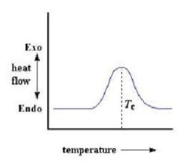
The temperature at the highest point in the peak is usually considered to be the polymers crystallization temperature, or Tc
