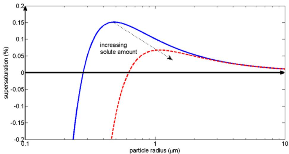
Figure 2: Köhler curve for two drops:  $m_s = 1 \times 10^{-17}$  g (blue solid line),  $m_s = 5 \times 10^{-17}$  g (red dashed line).
