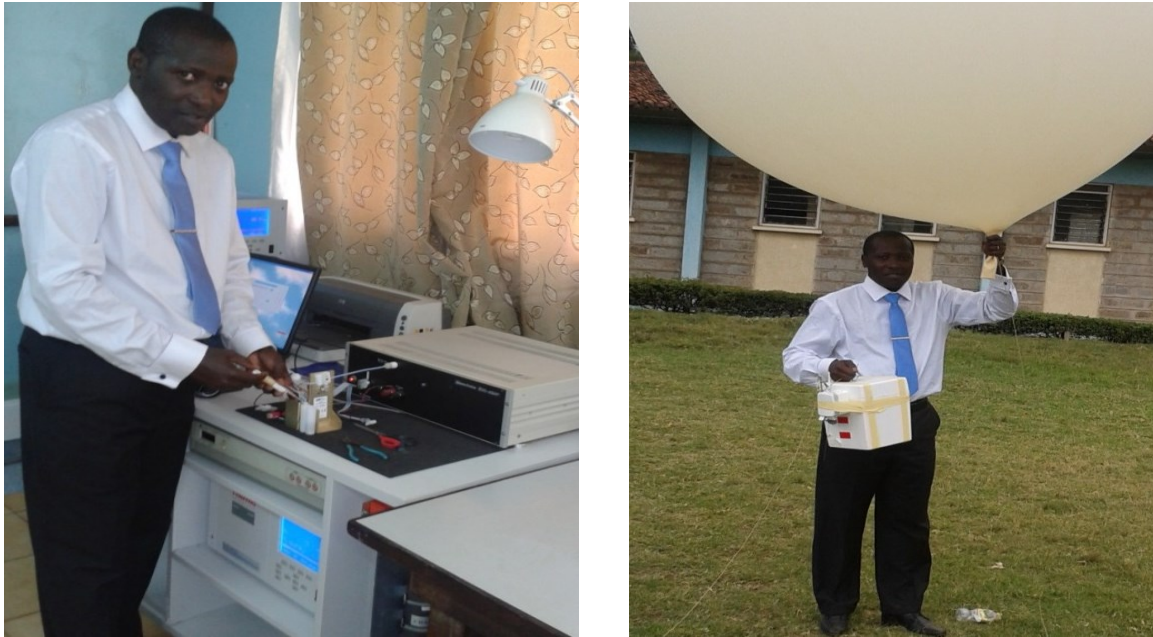
Figure 1; Scientist preparing the ozonesonde (left) and ready for flight (right)
