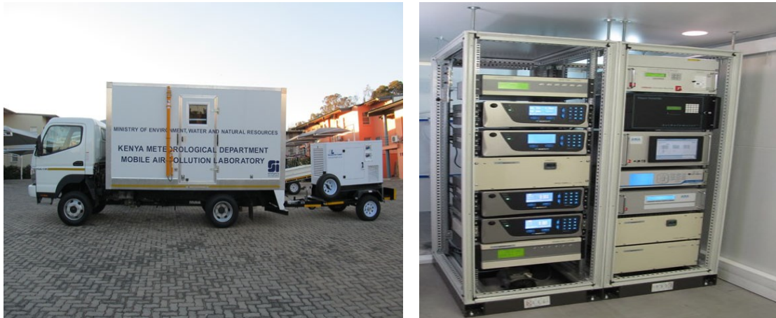
Figure 7; Mobile air van outside and inside showing the analysers,
