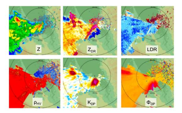
• Based on the values of the radar parameters a classification system is used to identified different types of hydrometeors
