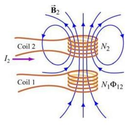
Changing current in coil 2 produces changing magnetic flux in coil 1.
