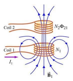
The first coil has  $N_1$  turns and carries a current  $I_1$  which gives rise to a magnetic field  $\mathbf{B}_1$ . Since the two coils are close to each other, some of the magnetic field lines through coil 1 will also pass through coil 2. Let  $\Phi_{21}$  denote the magnetic flux through one turn of coil 2 due to  $I_1$ . Now, by varying  $I_1$  with time, there will be an induced emf associated with the changing magnetic flux in the second coil:
