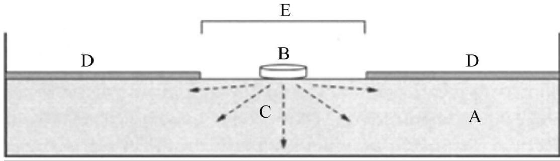
Disk sensitivity test. A – agar; B – antibiotic disc; C – antibiotic diffuses into agar along concentration gradient; D – bacterial growth on surface of agar after 18 hours of incubation; E – zone (diameter) of inhibition.
