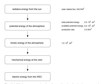
**Fig. 10.1.** Wind energy conversion flow diagram from irradiated solar energy to electric energy produced by a wind turbine. The values given for the energies and energy fluxes are long term global averages.
