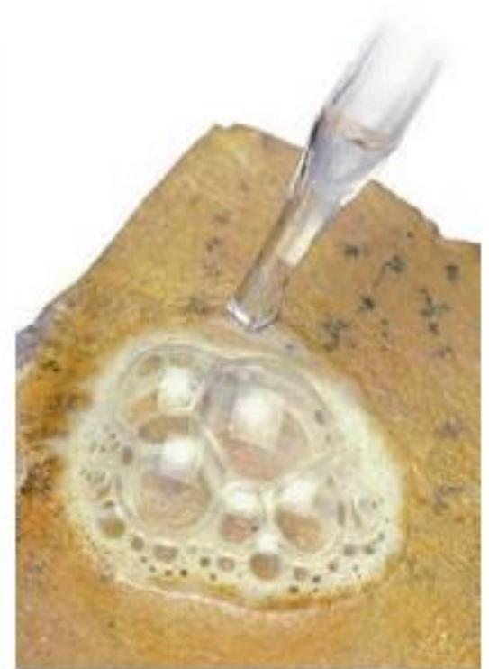
**Figure 3.21 Calcite reacting with a weak acid**
