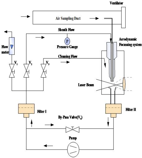
Fig. 1 - Aerosol sampling system
