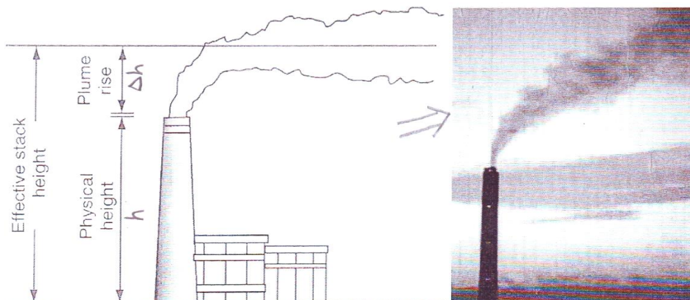
Figure (4-7): Chimney with initial specifications.
