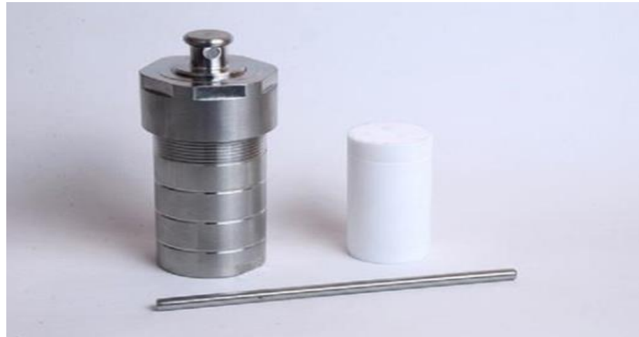
Figure (3) : Teflon lined autoclave.
