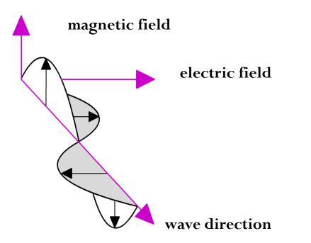
Electromagnetic waves are transverse waves made up of electric and magnetic fields
