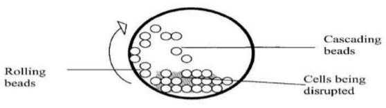
The basic principle of a bead mill
