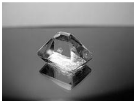
Potassium Alum Crystal with Unequal Distribution of the Octahedral Face Area
