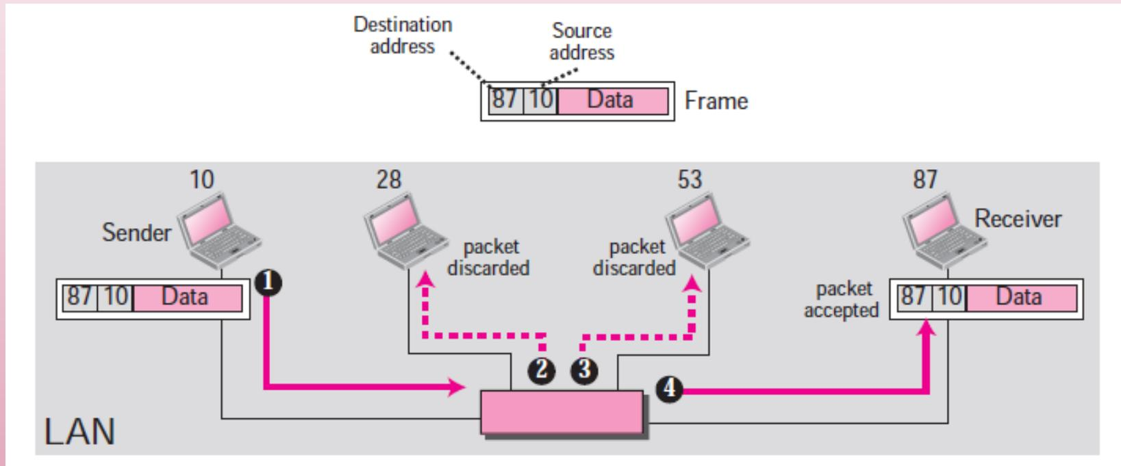
**Layer 2 addresses are only used to communicate between devices on a single local network**
