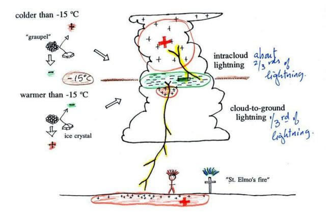
• When temperatures are colder than -15 C, graupel becomes negatively charged after colliding with an ice crystal. The ice crystal is positively charged and is carried up toward the top of the cloud by the updraft winds.
