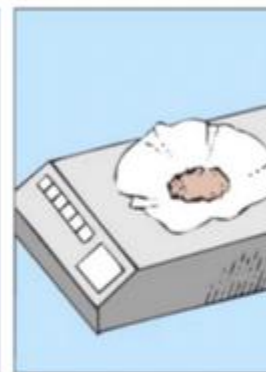
(e) Repeated drying and weighing until a constant mass of precipitate is obtained
