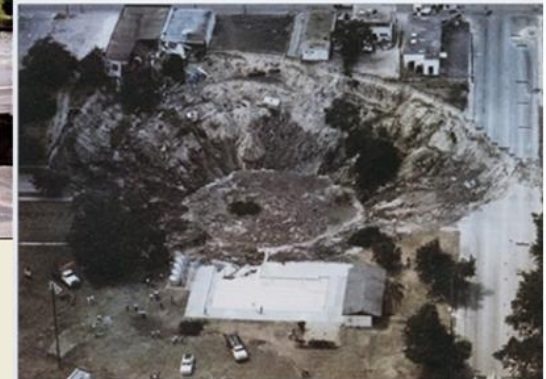
Figure 62. Spectacular, sudden collapse of the land surface commonly accompanies the formation of a sinkhole, such as this one that formed at Winter Park, just north of Orlando, Fla., in 1981.
