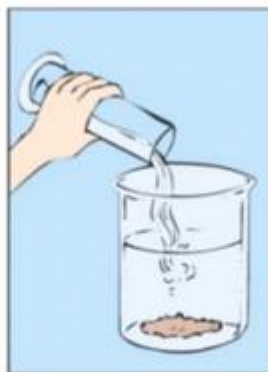
(c) Adding a suitable chemical to form a precipitate
