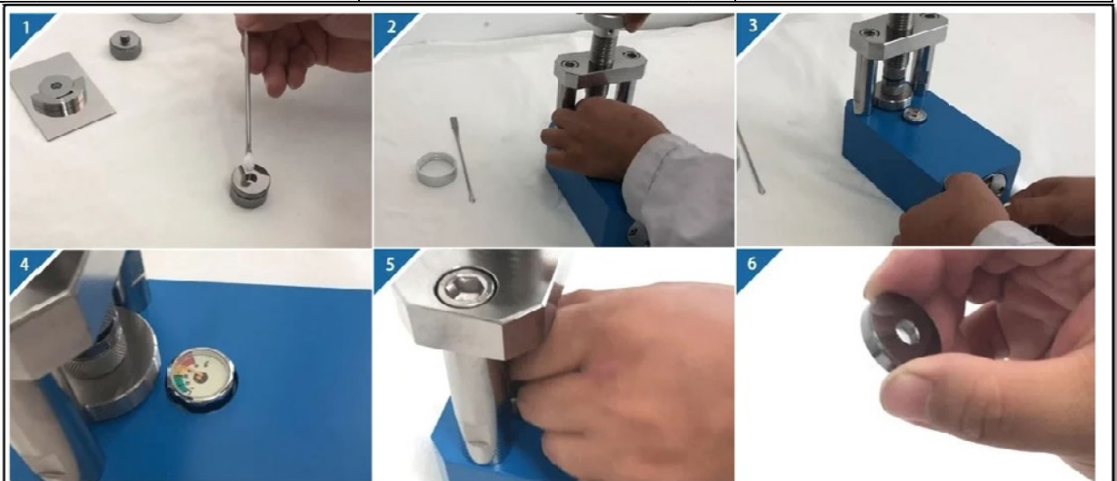
Preparation solid sample using KBr Pellet Press
