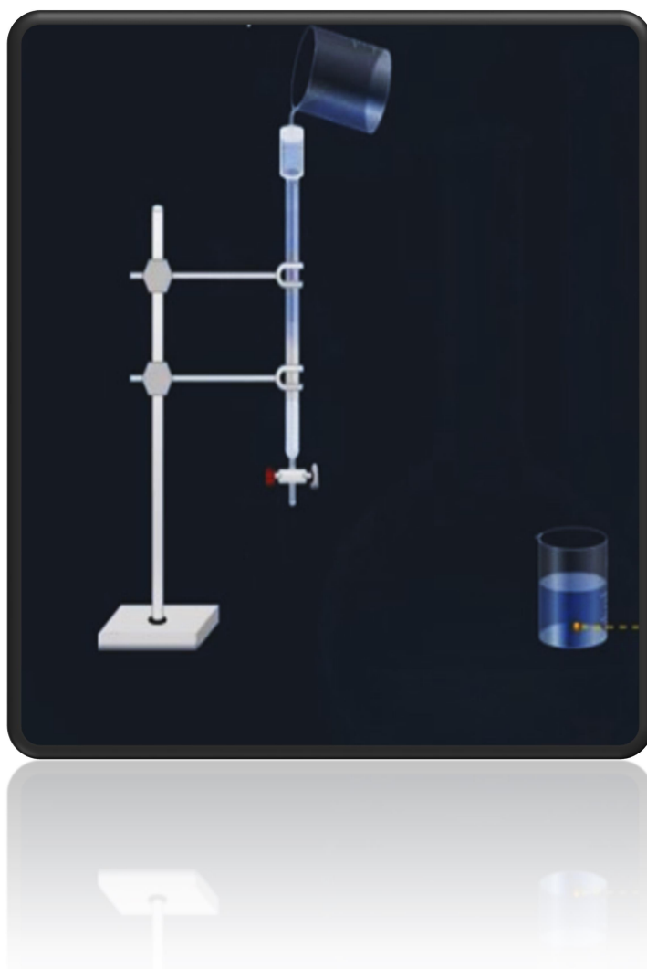
Figure (2) represents the addition of the mobile phase that was prepared with the first step and contains (NaCl + KCl) mixture to the previously activated ion exchange column.
