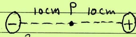
The diagram shows two point charges on a horizontal line. The left charge is negative, labeled  $-5 \times 10^{-8} \text{ C}$  with a circled minus sign. The right charge is positive, labeled  $+10 \times 10^{-8} \text{ C}$  with a circled plus sign. A point P is located between them, with dashed lines indicating a distance of 10 cm from each charge. The total distance between the charges is 20 cm.
