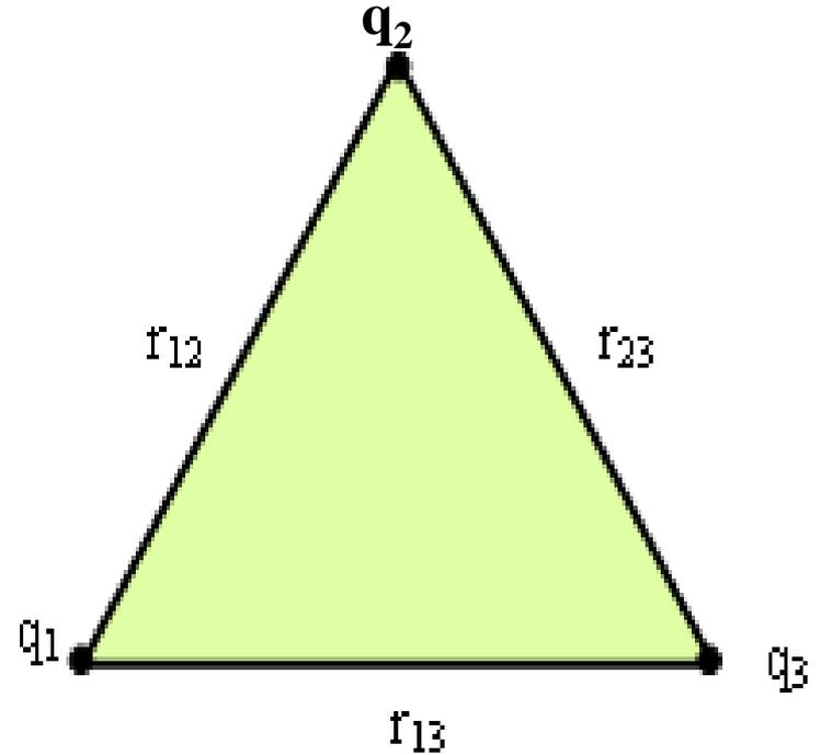
$$U = w_1 + w_2 + w_3 = \frac{1}{4\pi\epsilon_0} \left( \frac{q_1 q_2}{r_{12}} + \frac{q_1 q_3}{r_{13}} + \frac{q_2 q_3}{r_{23}} \right)$$
