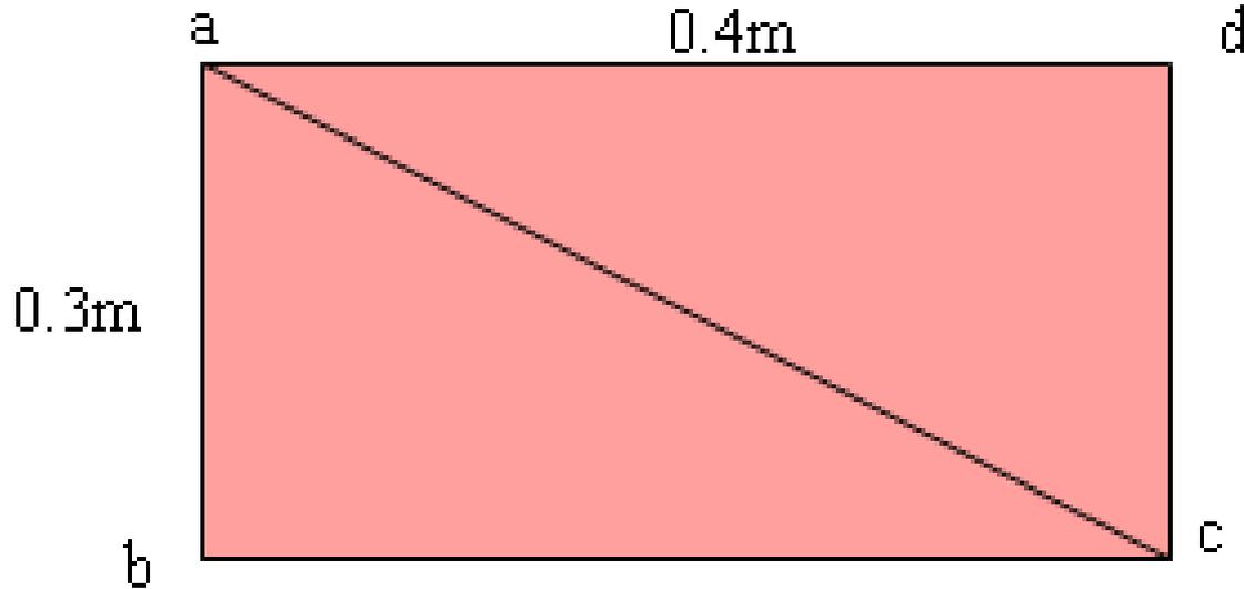
$$U = \frac{1}{4\pi\epsilon_0} \left( \frac{q_a q_b}{0.3} + \frac{q_a q_c}{0.5} + \frac{q_a q_d}{0.4} + \frac{q_c q_d}{0.3} + \frac{q_b q_d}{0.5} + \frac{q_b q_c}{0.4} \right)$$
