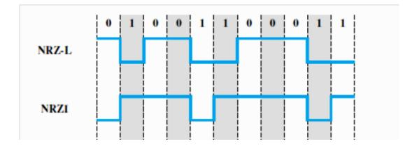
The main limitations of NRZ signals are the presence of a dc component and the lack of synchronization capability. To picture the latter problem, consider that with a long string of 1s or 0s for NRZ-L or a long string of 0s for NRZI, the output is a constant voltage over a long period of time. Under these circumstances, any drift between the clocks of transmitter and receiver will result in loss of synchronization between the two.
