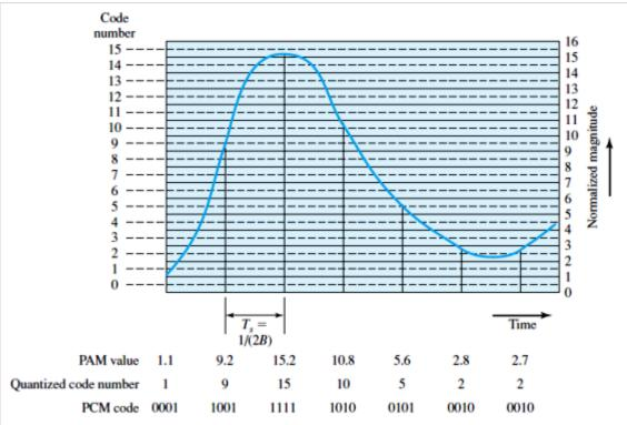
Figure 5.16 Pulse Code Modulation Example
