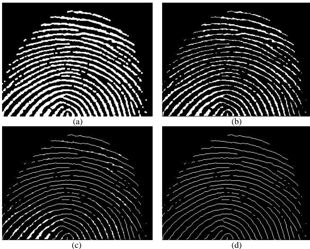
Figure 12.4 (a) Original fingerprint image. (b) Image thinned once. (c) Image thinned twice. (d) Image thinned until stability (no changes occur).
