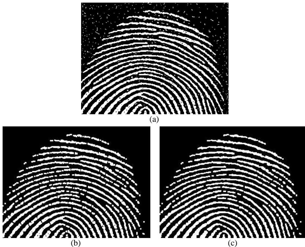
Figure 11.8 (a) Noisy fingerprint. (b) Result of opening (a) with square structuring element of size 3 pixels. (c) Result of closing (b) with the same structuring element.
