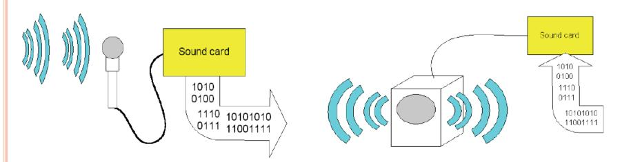
Take analog signals from analog sensor (e.g. microphone) and digitally sample data
