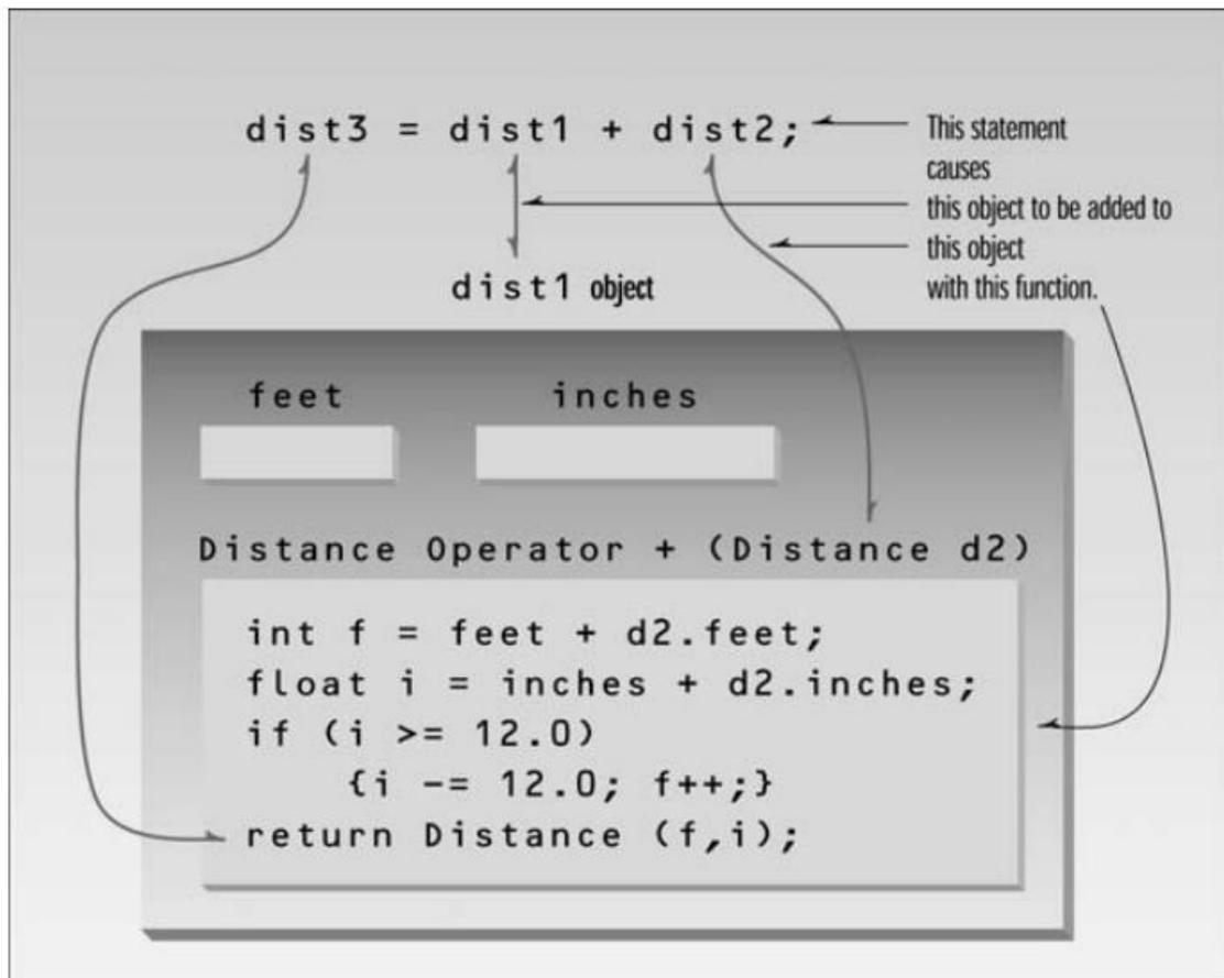
In the operator`+`(`)` function, the left operand is accessed directly—since this is the object of which the operator is a member—using `feet` and `inches`. The right operand is accessed as the function’s argument, as `d2.feet` and `d2.inches`.
