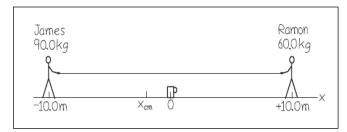
$$x_{CM} = \frac{m_1 x_1 + m_2 x_2}{m_1 + m_2} \qquad \Rightarrow \qquad x_{CM} = \frac{(90 \text{ kg})(-10 \text{ m}) + (60 \text{ kg})(10 \text{ m})}{(90 \text{ kg} + 60 \text{ kg})} = -2 \text{ m}$$
