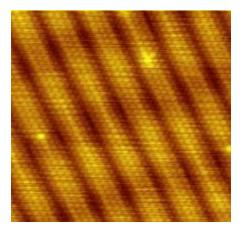
Image of reconstruction on a clean gold surface, as visualized using scanning tunneling microscopy. The positions of the individual atoms composing the surface are visible.
