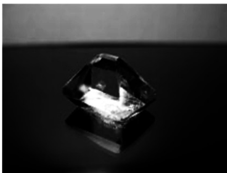
Potassium Alum Crystal with Unequal Distribution of the Octahedral Face Area
